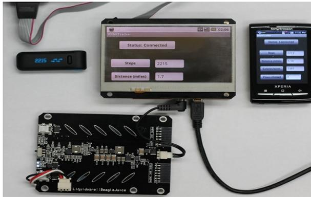
**Fig. 6.** Snapshot of testbed for FitLock, consisting of BeagleBoard and Xperia devices used as Fitbit trackers.
