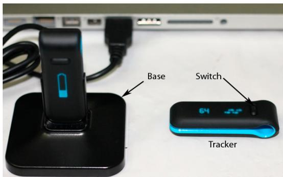
**Fig. 1.** Fitbit system components: trackers (one mounted on the base), the base (arrow indicated), user laptop. The arrow pointing to the tracker shows the switch button, allowing the user to display various fitness data.
