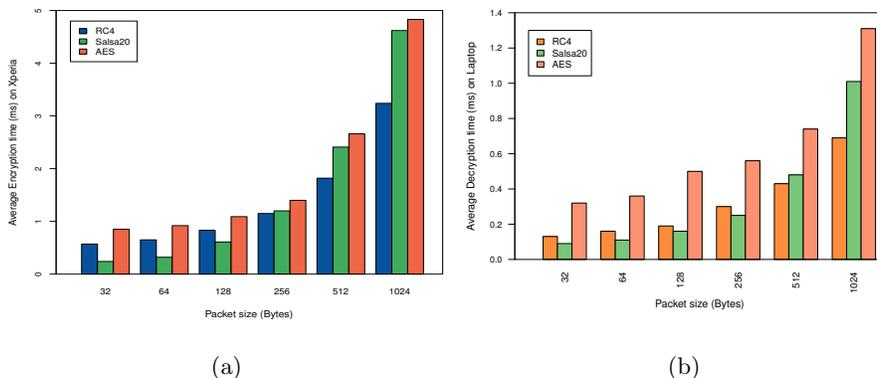
**Fig. 7.** FitLock overhead. (a) Encryption time overhead on Xperia. (b) Decryption time overhead on webserver (Dell laptop).
