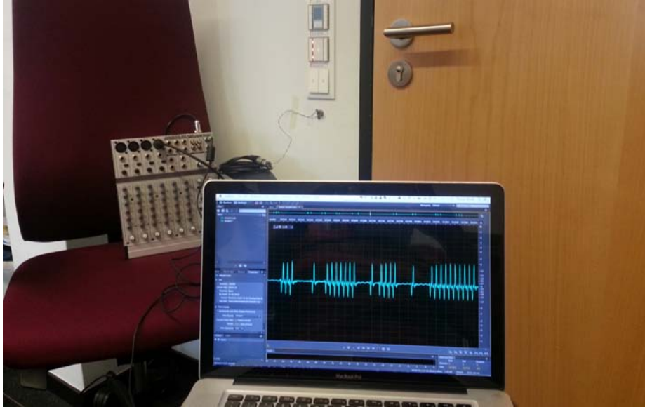
Fig. 9. Test setup with coil next to the wall switch, audio mixer used as pre-amplifier, and a notebook with audio input and recording software.
