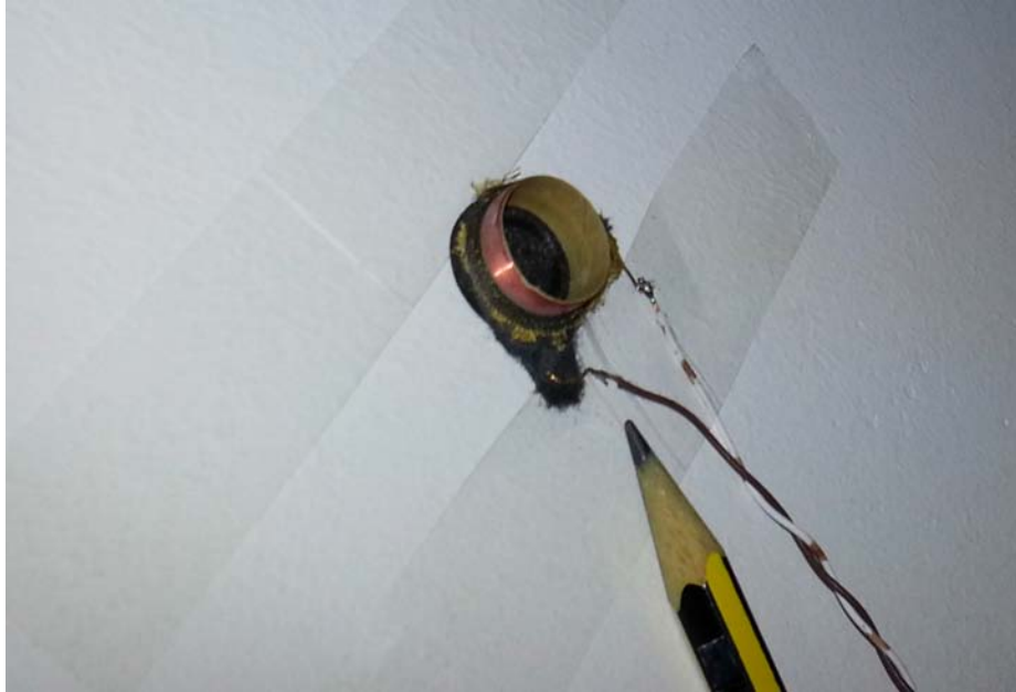
Fig. 11. A coil taken from a loudspeaker. The magnetic core has been dismantled to build an air loop antenna.
