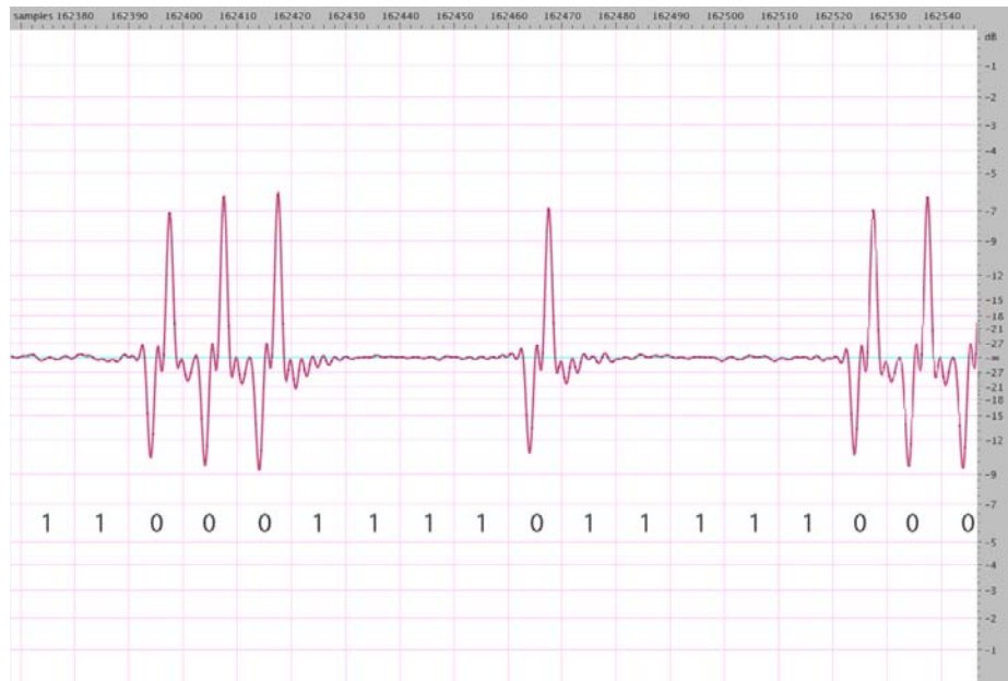
Fig. 10. Wave form as recorded and decoded bit values. Note that KNX on two wire Twisted Pair cables uses a constant voltage to indicate a logical “One” and a “peak” to indicate a logical “Zero”. There is no clock signal, but the protocol guarantees frequent “zeros” for synchronization.
