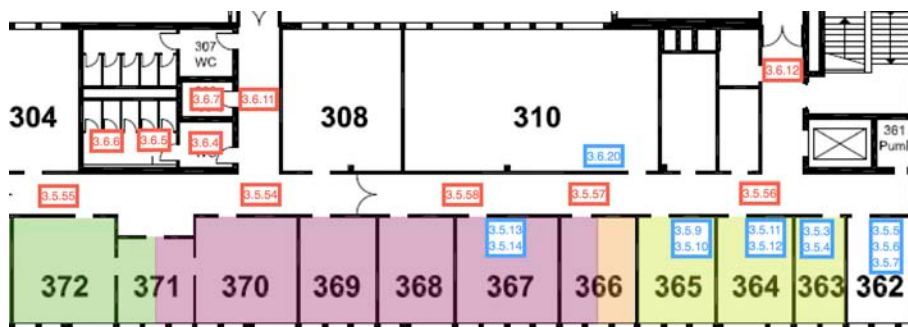
Fig. 7. Sample floor plan with addresses of some sensors. Infrared presence detectors are marked in red, switches in blue.
