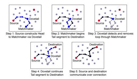
Fig. 2. Construction of a Dovetail connection
