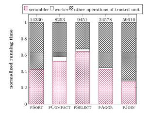
**Fig. 3.** Normalized running time breakdowns for STC's algorithms. The total running time (in seconds and displayed on top of each bar) comprises of the time taken by the scrambler, by the worker, by the pre-processing and post-processing steps, and by the main algorithm logic.
