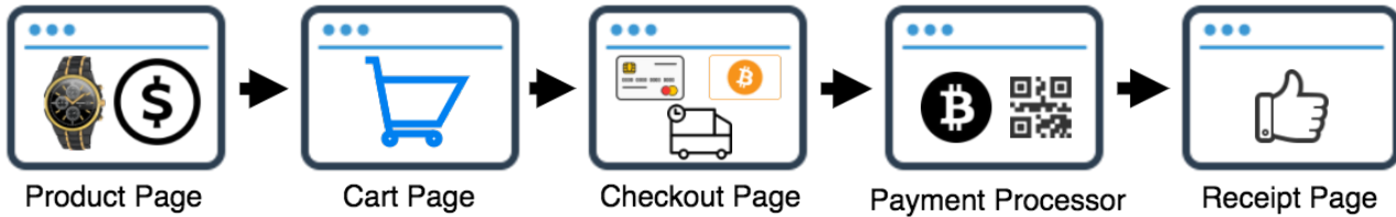
Fig. 2. An illustration of a typical payment flow on a merchant site. Each step of this flow presents opportunities for leaking transaction-relevant information to embedded third-party trackers.
