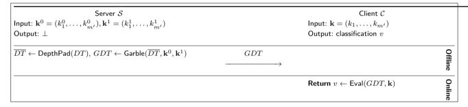
Fig. 11. Path<sub>G</sub> - Oblivious path evaluation using a garbled decision tree.
