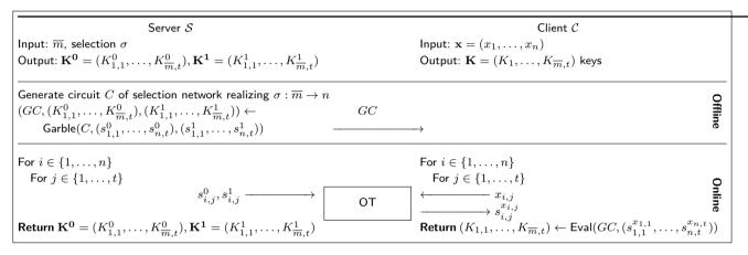
Fig. 7. Sel<sub>G</sub> - Oblivious selection using a garbled selection network.
