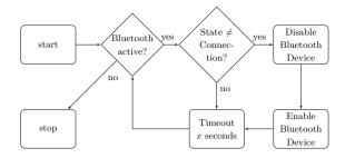
**Fig. 14.** A proposed workaround which breaks tracking via the address-carryover algorithm on Windows 10 and iOS/macOS devices.
