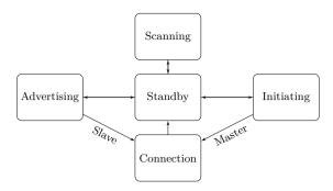
Fig. 1. The Link Layer State machine [20, p. 15]
