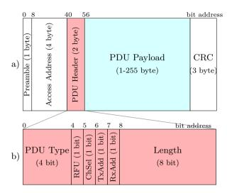
**Fig. 2.** The BLE advertising packet format (Fig. 2.a)) and the Advertising Channel PDU Header (Fig. 2.b)) [8, p. 2562, 2567].
