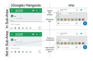
Fig. 8. Hangouts and imo had separate OSIs with Typical scope and Sub-Area scope showing other users' presence in a conversation
