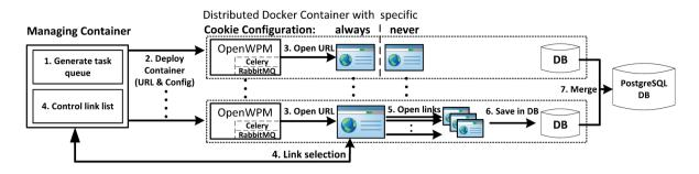
Fig. 2. Experimental set-up
