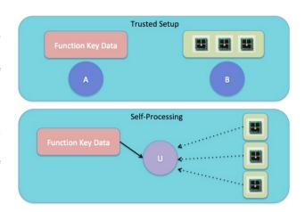
Fig. 1. The two steps of a self-processing sensor data scheme. First, there is the trusted setup after which A has function key data and B has sensors. Once B deploys the sensors, any user U with access to the function key data can monitor the sensor broadcasts and learn the function evaluations.
