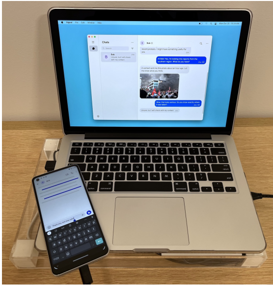
(a) The internet-connected smartphone is connected to the air-gapped laptop through a data diode. Messages received on the smartphone can only be decrypted on the laptop. Data physically cannot leave the laptop, since its wireless radios, speakers, and USB ports are disabled: the laptop can only receive data through the data diode. Each device shows Signal user interface mockups.
