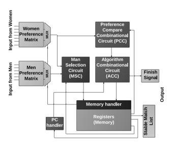
**Fig. 4.** Block diagram architecture of the sequential circuit for implementing secure SM.
