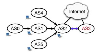
**Fig. 1. Topology-based attacks**. AS3 is a compromised AS and receives a packet form AS2 and conducts topology-based attacks to de-anonymize the packet's source node. The arrow from an AS points to its provider and the relationship between AS2 and AS3 can be peer-to-peer, customer-to-provider, and provider-to-customer.
