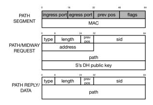
Fig. 7. Formats of a path segment and packet headers. The shaded fields are encrypted using a node's local secret key.
