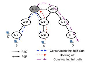
**Fig. 4. Back-off path setup**. The arrow standing for P2C relationship always points from the provider to its customer. The shaded node is the midway node. We call the path between S and M the first "half path" and the one between M and D the second "half path".
