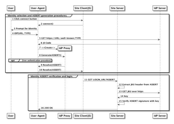
Fig. 7. Identity assertion management sequence diagram.
