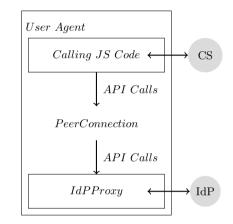
Fig. 4. WebRTC Identity Architecture
