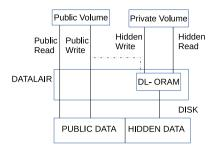
**Fig. 5.** Design of DataLair *Lite*. Writes to the hidden partition happen through DL-ORAM.
