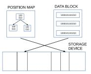
Fig. 1. DL-ORAM. The position map blocks are randomly interleaved with the data blocks within the same address space.
