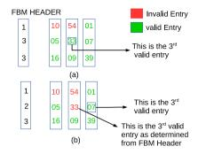
Fig. 3. Example of FBM with 9 entries. In (a), the FBM header correctly determines that the  $3^{rd}$  valid entry is at (2,2) since there is 1 valid entry in the first row and 3 in the second. In (b), the  $3^{rd}$  valid entry is determined incorrectly since the FBM header correctly indicates that the second row has 2 valid entries but does not show which columns have the valid entries.
