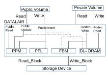
Fig. 8. DataLair full design with the four main components: DL-ORAM, PPM, PFL and FBM. Hidden data I/O is mapped through DL-ORAM while public data I/O is mapped through the PPM. The public data inserts and updates simulates an access to the DL-ORAM. In  $ONLY\_PUB$  mode free blocks are located using the PFL.
