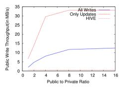
**Fig. 9.** Variations in public write throughput vs. the public write to private write ratio. The x-axis represents the number of public writes that are performed in between two private writes/simulation. The throughput plateaus at around 12~MB/s, around 6x faster than the configuration where hidden writes are made with each public write. The benefits of performing hidden writes only with updates is visible even in this case.
