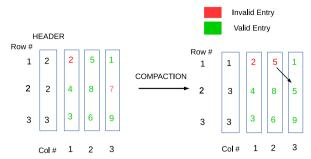
Fig. 4. Compacting the FBM. Invalid entries appear before valid entries when entries are traversed *row-wise*. In the example, 7 was selected randomly from (2,3) which was replaced by 5 from (1,2) to ensure compactness.
