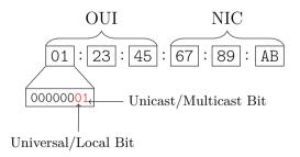
Fig. 1. 48-bit MAC Address Structure
