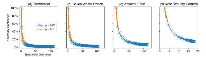
Fig. 4. STP tradeoff between bandwidth overhead and adversary confidence for different devices and user activity frequencies p. Each point corresponds to a probability of non-activity padding q ranging from 0 (highest adversary confidence) to 1 (highest bandwidth overhead) in steps of 0.01. Note the inverse square relationship, which allows STP to achieve low adversary confidence for relatively little bandwidth overhead.
