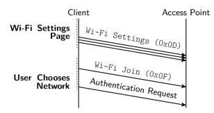
Fig. 6. Wi-Fi Join – Authentication Frame Global MAC Exposed
