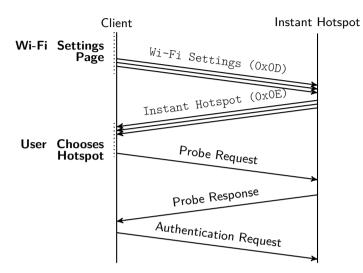
Fig. 4. Instant Hotspot Discovery and Connection Setup
