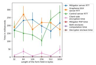
Fig. 7. An identical setup to that in Figure 5, with the exception that requests are sent from a browser extension, instead of a headless client, on another remote machine with higher network latency, and n = 10 requests are sent for each data point. The bottom three lines are all indistinguishable at the bottom of the graph.
