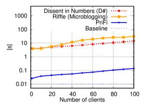
(b) Latency comparison between PriFi, D# and Riffle, computed as the time to send and decode an anonymous message. The baseline is the latency of the LAN (10 ms).
