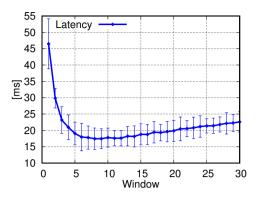
Fig. B.5. Effect of pipelining on latency. A window  $W\!=\!7$  divides the latency by 2.25 in comparison to the naı̈ve  $W\!=\!1$  approach.
