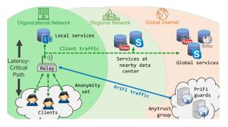
**Fig. 1.** PriFi's architecture consisting of clients, a relay, and a group of anytrust servers called the *guards*. Clients' packets remain on their usual network path without additional hops, unlike in mix-networks and onion-routing protocols.
