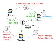
Fig. 2. Example of a 1-bit DC-net.
