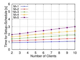
$\label{eq:Fig.B.8.} \textbf{B.8.} \ \ \text{Duration of } \ \ \text{Setup. This corresponds to the downtime in } \\ \text{case of client churn.}$
