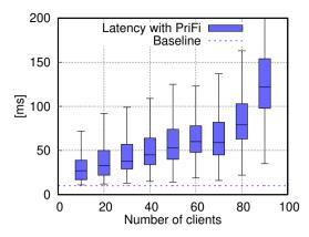
(a) Latency increase when using PriFi. The baseline is the latency of the LAN (10 ms).
