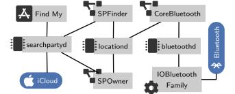
Fig. 3. Simplified view of components and their interactions such as apps (☑), daemons (♣), frameworks (☜), and drivers (✿) that are used by OF on iOS. We highlight the two involved external communication interfaces in blue.
