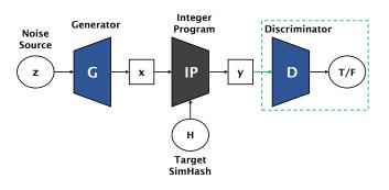
Figure 3: Pipeline: integer programming on the generator outputs. The green boxed part is optional.
