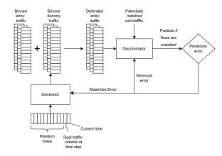
Figure 5: FC-DeTorrent Training, where the generator is trained to reduce the discriminator's ability to predict which flows are matched. The discriminator is trained to determine which flow pairs are associated with the same connection, and the generator is trained to defend the traffic to prevent this.
