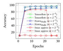
Figure 9: Accuracy comparison of PPNN training on MNIST. Here  $\alpha$  denotes learning rate and for HAWK<sub>Multi</sub>,  $\epsilon_T = 0.1$ . The Softmax approximation used by past works causes accuracy drop.
