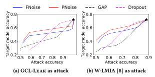
Figure 17: Target-attack trade-off of the defense mechanisms against GCL-Leak and W-LMIA [8] (GRACE model, Citeseer dataset, r=0.4 for PNoise).  $\star$  indicates no defense.
