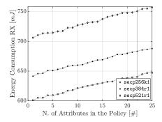
Figure 11: Energy required for messages verification and decryption through SNELL, increasing the number of attributes into the access control policy, with various elliptic curves.
