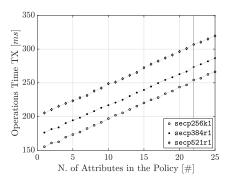
Figure 8: Messages generation time through SNELL, increasing the number of attributes into the access control policy, with various elliptic curves.
