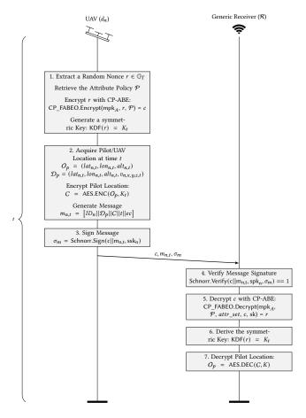
Figure 3: Sequence Diagram of the *Deployment Phase* of SNELL.
