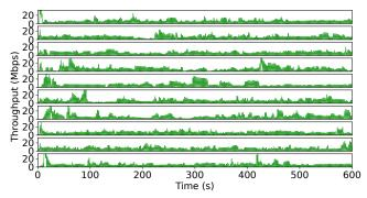
Figure 1: Throughput of 10 video streams using MPEG-DASH
