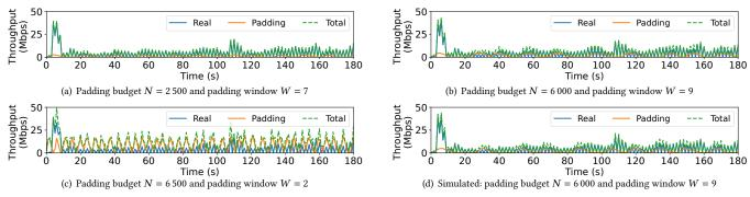
Figure 11: Throughput using Adapted FRONT collected over physical machines (a-c) and via simulation (d)
