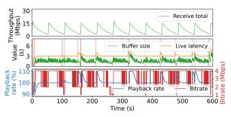
Figure 26: Throughput and video player QoE metrics using Adapted RegulaTor with  $R_0 = 1\,900$  and D = 0.95
