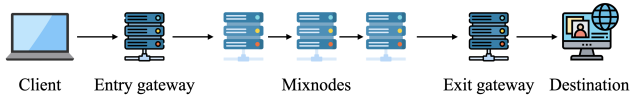
Figure 1: A typical communication path in the Nym mixnet. Note that NymVPN “fast mode” omits the mixnodes.
